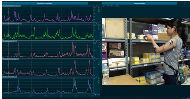
Sample test of muscle exertion levels associated with bar code scanning
